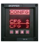
Placing TXT in the bottom 4<sup>th</sup> line or 3<sup>rd</sup> and 4<sup>th</sup> line will cause the data to spread out showing fewer data points. The system will not allow you to mix speed data from different sources on the same screen. Having 2 TXT lines after each other will also rearrange the positioning.
